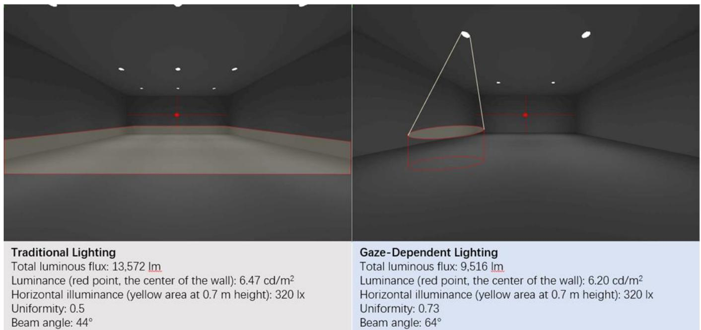
**Figure 1: Simulation images for conventional illumination (left) and gaze-dependent illumination (right).**
