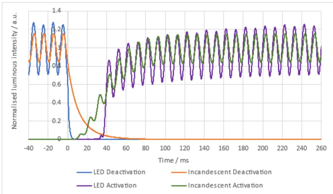
**Figure 1: Example activation and deactivation profiles of LED vs incandescent traffic signals, showing that there can be a time for the LED signal colour transition where no signal is visible.**
