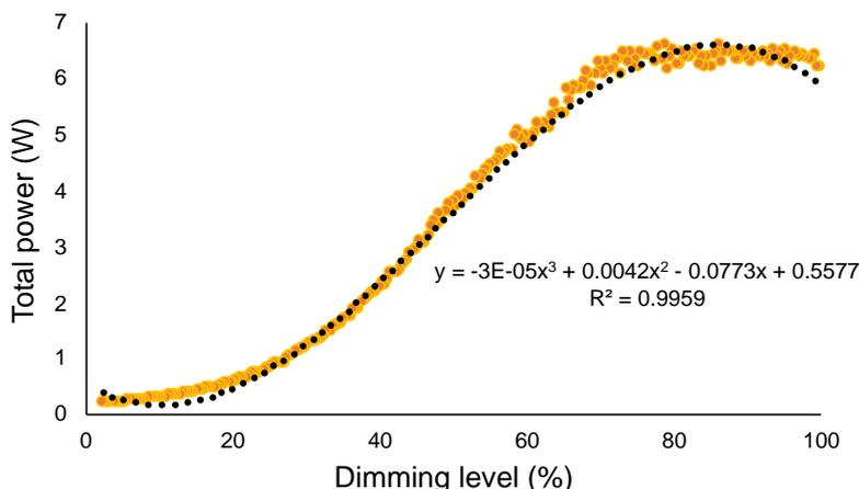
**Figure 1: The cubic fitting (black dotted line) of the total measured power of a blue LED (y-axis) to dimming levels (x-axis)**
